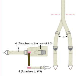
Trim belt here if using Airfix supplied seat and if no cutout is made.
