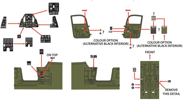
NOTE: Some areas such as the main instrument panel need to be sanded smooth to get best application of decal. Use of PVA or decal fix is advised to stick decal in place (due to the thicker nature of the printing technique the standard decal sheet adhesive may not be adequate to hold the decal in place).
